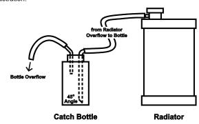
Overflow tube exiting the catch can must be routed to the rear of the motorcycle and configured so as to discharge onto the exhaust or muffler.
